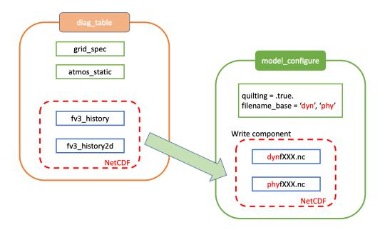
Fig. 4.1: Relationship between diag\_table, model\_configure and generated output files
